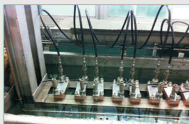
Pressure Leakage Test
