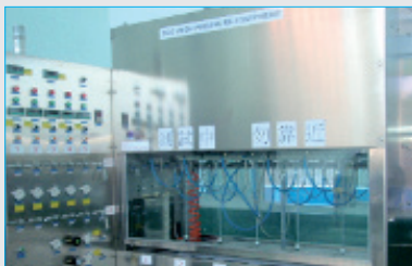
CO 2 High Pressure Test
